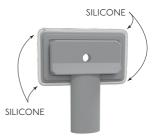
Apply a bead of silicone around all four sides of the rear overflow cover (externally) or reposition as needed to achieve a snug fit and a waterproof seal.
